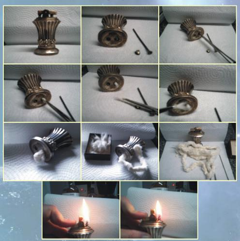
In the first you can see how it was when it arrived. In the second photo, I have removed the two screw caps on the base, the flint holder and petrol filling hole.
